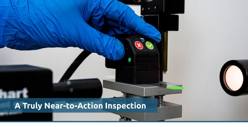
The quantitative inspections of the Surface Analyst are the first step to understanding your adhesion and cleaning processes. The portability and ease-of-use of the Surface Analyst 5001 device allows users to walk their production line to inspect material surfaces and map **Critical Control Points**—areas within production where surface condition has the opportunity to change and impact adhesion and cleaning outcomes.
